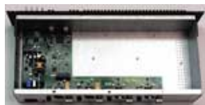
Figure 6: Closed steel pan shields front panel controls.
